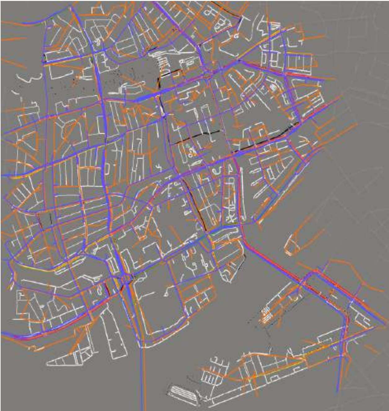
Figure 16. Graph networks of Rotterdam study area with import of the microscopic network model in Paramics software (blue) and macroscopic network model in OmniTRANS software (orange)
